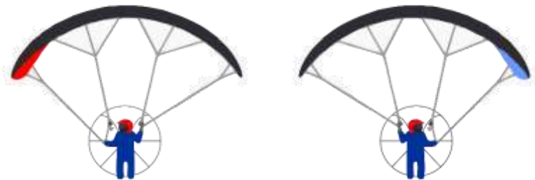
FAST and SUPER-FAST- 2D tip steering ONLY 2D tip steering line only
